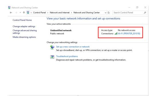
When the printer is set to the default value (Soft-AP mode, SSID: PRINTER\_XXXXXX), it will automatically connect.
