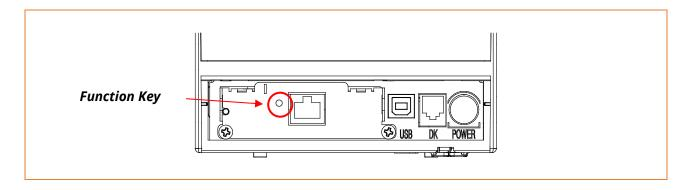
With the printer turned off, press the function key button and turn the printer on. After pressing and holding the function key button for about 5 seconds, release it. The factory reset occurs. Regardless of the current setting, DHCP mode is enabled.
